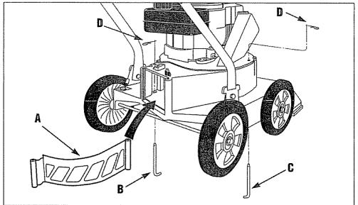
Figure 3: Shredder screen installation.
